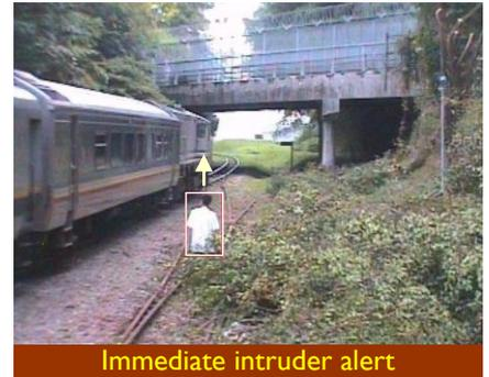
Additional features are available to minimize false positive. External interferences such as reflections of raindrops, changes in brightness and background in outdoor environment; are being filtered out in the detection and tracking processes. One example is the tracking and sending of immediate alarm when human-like objects are confirmed walking among moving vehicles in restricted zone of busy multi-lane motorway.
